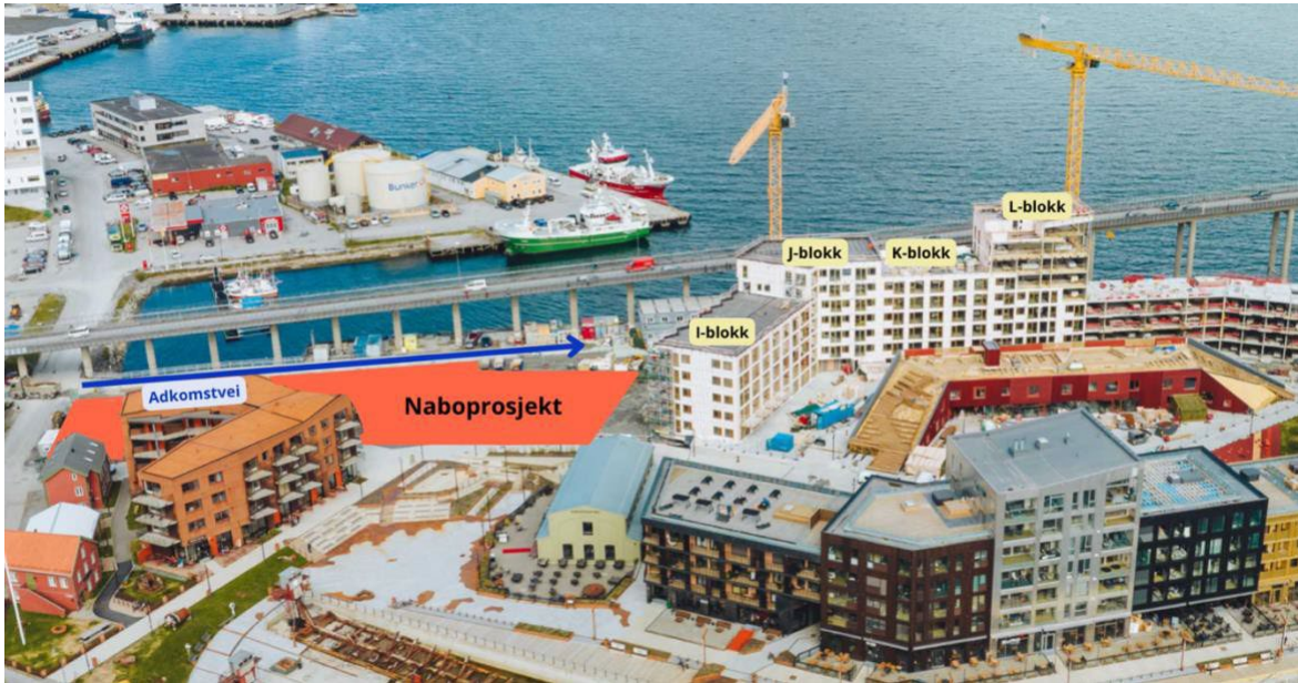
Figure 6: Access road (dark blue) to the construction site and construction activity on the neighboring plot (orange). (Drone image used with permission from Vegard Stien.)
